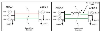
seeks to flow through that line in preference to the other (left part of the diagram). By installing PLGs on the upper line, impedance can be increased, balancing out power flows on the two lines (right part of the diagram) thus utilizing the total available transmission capacity.
