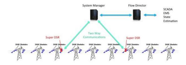
In addition to controlling PLGs, the communications capabilities allow PLGs to provide real time data on the lines including: line current, conductor temperature, frequency, sag and blowout angles, PLG status and PLG set point. Fault indication provides information of where a fault occurred (between which two PLGs). Other optional capabilities include conductor vibration and geomagnetic induced current detection.
